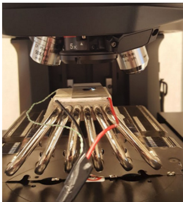
Figure 1. Bituminous sample placed on the in-house heating element under CLSM.
